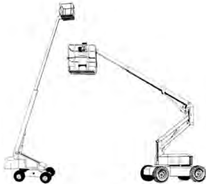
Figure 22-3: Boom-Type Powered Platforms
