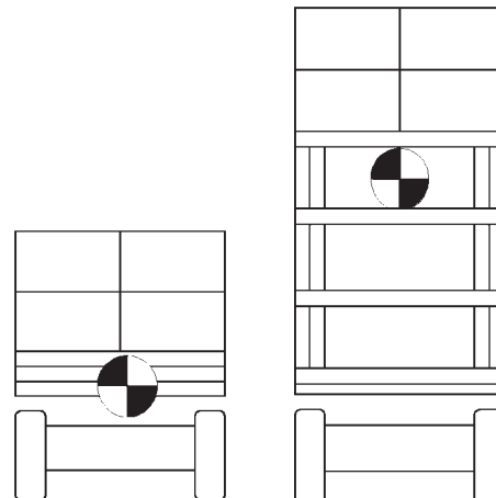
Figure 22-8 Centre of Gravity on Scissor-Type Lifts
